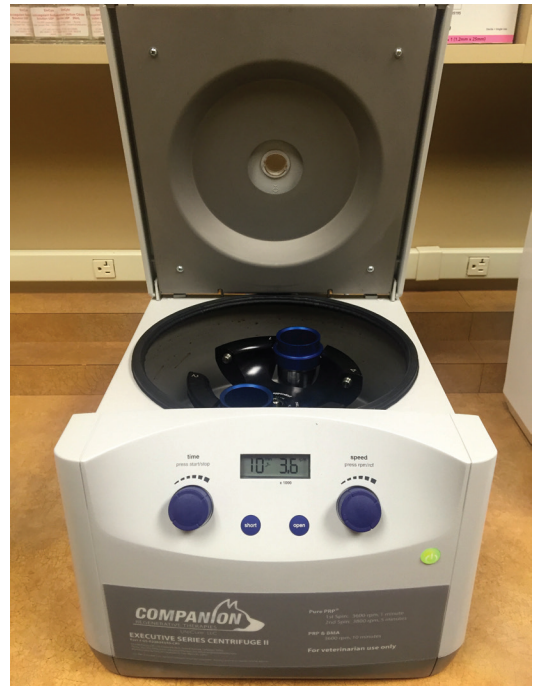
FIGURE 2. Both centrifugation and filtration systems are available for PRP processing. This centrifugation PRP system used for processing produces a leukocyte- and erythrocyte-poor PRP sample.
